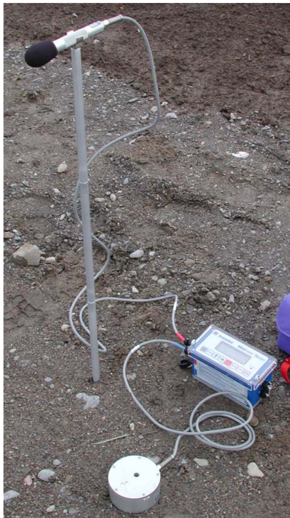
Figure 1 Installing the Minimate Blaster.
