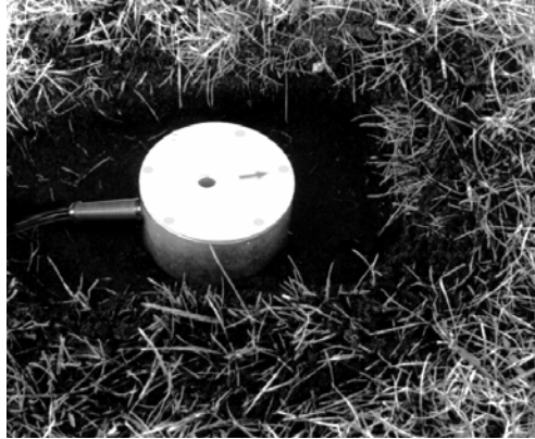
Figure 7 Burying the Standard Transducer.
