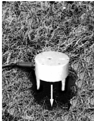
Figure 5 Installing the Standard Transducer using the Ground Spikes.
