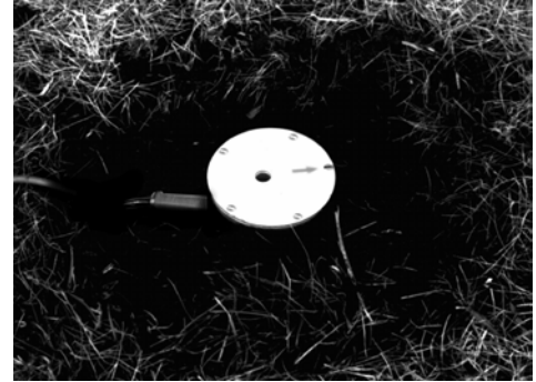
Figure 8 Fill in and pack the material around the Standard Transducer.
